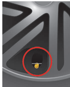
Incorrect valve position: below the ring.
