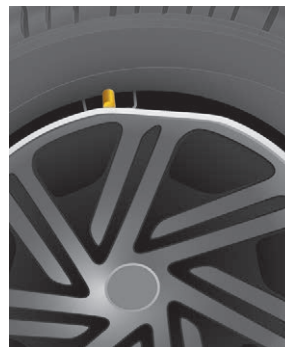
Distortion of the edge of the wheel trim at the valve due to incorrect fitting.
